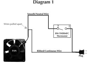
When using one fan, the fan should blow into the enclosure.
